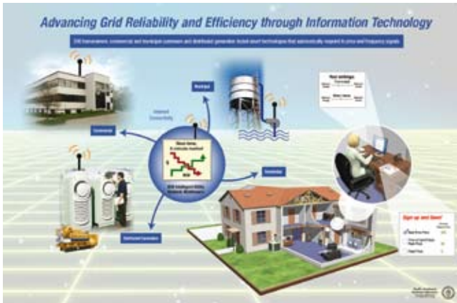
Demand response programs help limit energy use at specific peak times, when demand strains the electric grid and increases costs for both utilities and customers.
